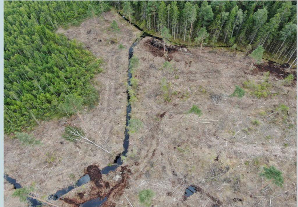
Figure 3: Small rewetting measures with artificial beaver dams. Left: single measure, right: combination of several measures.
