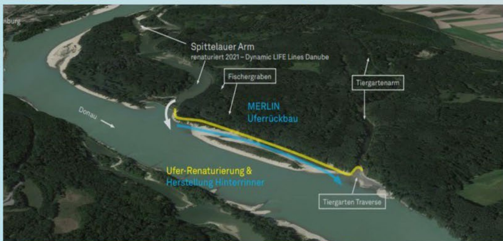
Figure 4: River stretch for removal of river bank fixation and restoration of the river bank.
